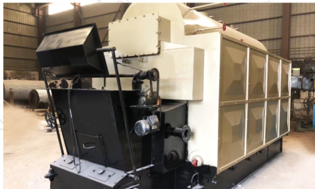
2018.04.28 河南永乐粮油机械有限公司2吨生物质蒸汽锅炉 2018.04.28 2t/h biomass fired steam boiler in Henan Yongle Cereals and Oils Machinery Co.Ltd
